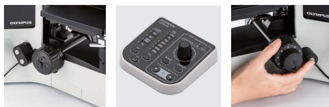
Hand switch for motorized nosepiece rotation
